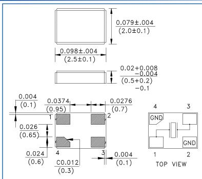
**Note:** From the top view (marking side), pin #1 is always located at the bottom left corner of the package. This is regardless of the location of the Chamfer, since due to material availability, the Chamfer could be located on pin#1, 2 or 4. Be advised that the Chamfer location has no impact on the electrical performance of the device.
