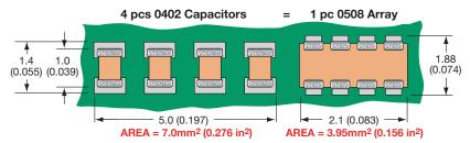
The 0508 4-element capacitor array gives a PCB space saving of over 40% vs four 0402 discretes and over 70% vs four 0603 discrete capacitors.
