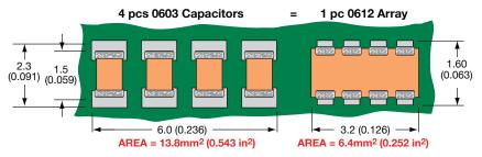
The 0612 4-element capacitor array gives a PCB space saving of over 50% vs four 0603 discretes and over 70% vs four 0805 discrete capacitors.
