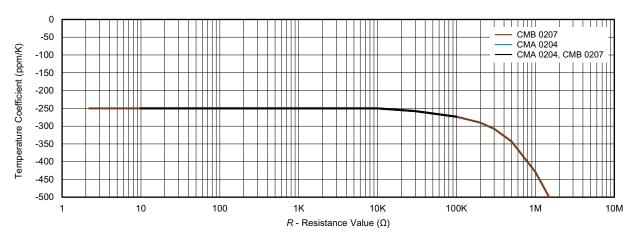
Typical curve for carbon film according to applicable resistance value range
