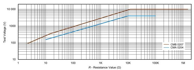
Pulse load rating in accordance with IEC 60115-1, clause 4.27; 1.2  $\mu$ s / 50  $\mu$ s; 5 pulses at 12 s intervals; for permissible resistance change  $\pm$  (0.5 % R + 0.05  $\Omega$ )
