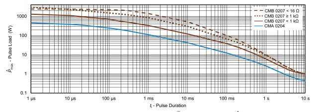
Maximum pulse load, single pulse; applicable if  $\bar{P} \to 0$  and n  $\leq 1000$  and  $\hat{U} \leq 4$  kV (CMB); or  $\hat{U} \leq 2$  kV (CMA); for permissible resistance change  $\pm$  (0.5 % R + 0.01  $\Omega$ )
