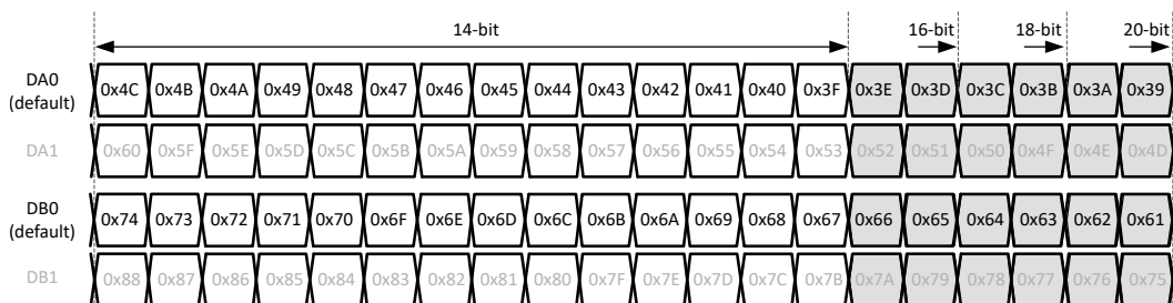
Figure 8-38. 1-wire output bit mapping
