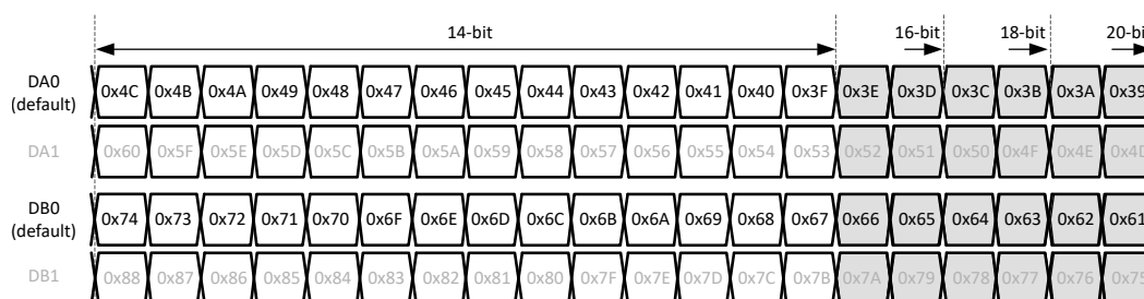
Figure 8-44. 1-wire output bit mapping
