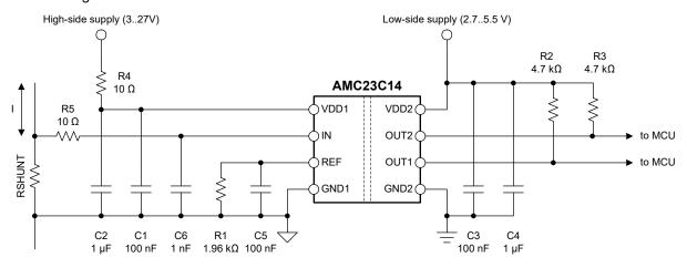
Figure 8-9. Decoupling of the AMC23C14
