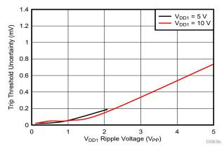
Figure 8-6. Trip Threshold Sensitivity to VDD1 Ripple Voltage (Cmp1, f<sub>RIPPLE</sub> = 10 kHz)
