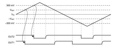
Figure 6-2. Functional Timing Diagram
