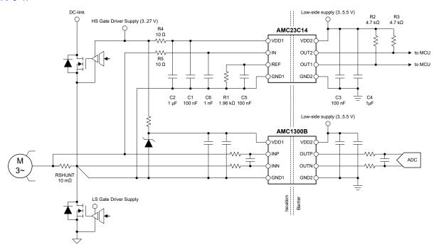
Figure 8-1. Using the AMC23C14 for Overcurrent and Short-Circuit Detection
