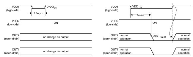
Figure 7-11. Output Response to a Short Brownout Figure 7-12. Output Response to a Long Brownout Event on VDD1 Event on VDD1
