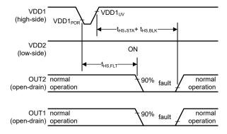
Figure 7-13. Output Response to a Power-Loss Event on VDD1
