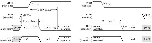
Figure 7-7. VDD2 Turns On, Followed by VDD1 (Short Delay)
