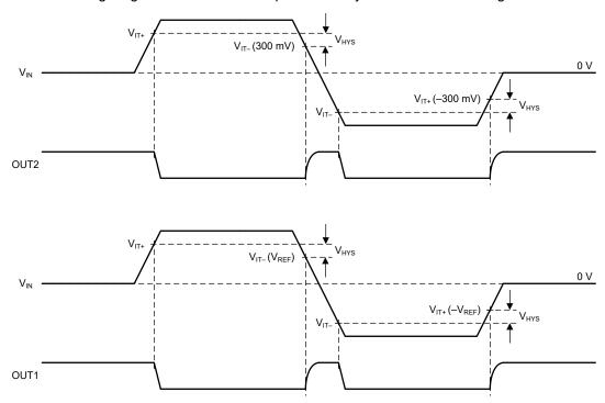
Figure 7-1. Switching Thresholds and Hysteresis
