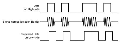
Figure 7-4. OOK-Based Modulation Scheme
