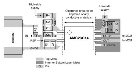
Figure 8-10. Recommended Layout of the AMC23C14
