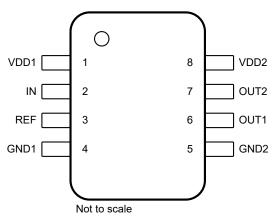
Figure 5-1. DWV Package, 8-Pin SOIC (Top View)
