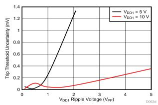
Figure 8-7. Trip Threshold Sensitivity to VDD1 Ripple Voltage (Cmp2, f<sub>RIPPLE</sub> = 10 kHz)
