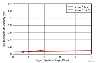
Figure 8-5. Trip Threshold Sensitivity to VDD1 Ripple Voltage (Cmp0, f<sub>RIPPLE</sub> = 10 kHz)
