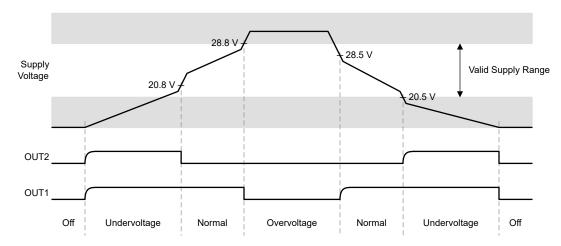
Figure 8-3. Output of the AMC23C14 in Supply Voltage Supervisor Application
