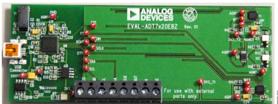
Figure 1. ADT7x20 Evaluation Board—Main Board
