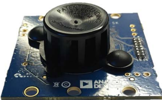
Figure 6. Evaluation Board Attached to Chamber, Side View
