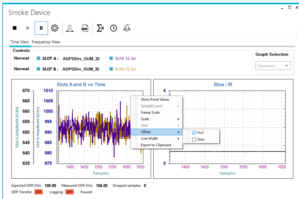
Figure 7. Null Background Response with the Wavetool Evaluation Software
