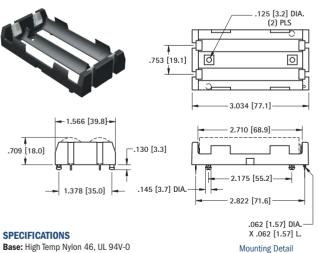
Base: High Temp Nylon 46, UL 94V-0 Contacts: .012 (.30) Stainless Steel, Tin-Nickel Plate
