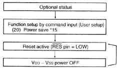
Set the time (tu) from reset active to turning off the VDD - Vss power (VDD - Vss = 1.8 V) longer than the time (th) when the potential of V<sub>5</sub> ~ V<sub>1</sub> becomes below the threshold voltage (approximately 1 V) of the LCD panel. For th, refer to the <Reference Data> of this event. When the is too long, insert a resistor between Vs and Vpp to reduce it.
