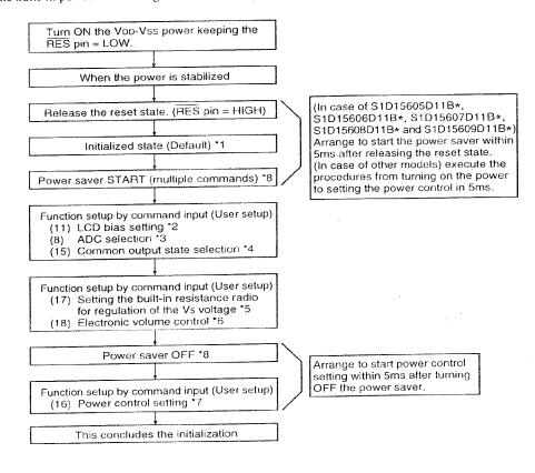
\* The target time of 5ms will result to vary depending on the panel characteristics and the capacitance of the smoothing capacitor. Therefore, we suggest you to conduct an operation check using the actual equipment.
