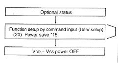
Set the time (fL) from power save to turning off the VDD - Vss power (VDD - Vss = 1.8 V) longer than the time (th) when the potential of  $V_5 \sim V_1$ becomes below the threshold voltage (approximately 1V) of the LCD panel. • this determined depending on the voltage
