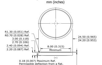
0.10 (0.004) Minimum Ref. (Applies to top edge of gasket or edge of crimp, whichever is higher.)
