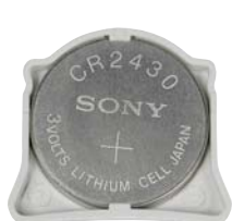
Insert Coin Cell into the Tray
